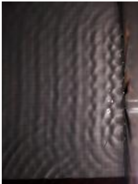
Figure 2. Talbot carpet for surface waves in liquid
