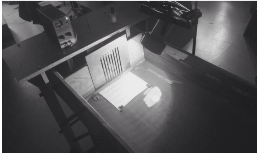
Figure 1. Scheme of experimental setup for observation of Talbot effect for waves on the liquid surface
